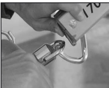
Easy opening of the carabineer by pushing the safety catch backwards with one finger and attachment of the spreader bar.
